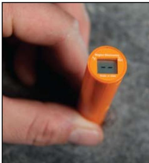
*Easy Reader* powering on after inserted into Smart Sensor
