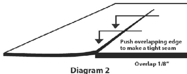
**NOTE:** Over compressing the seam will result in bond failure.
